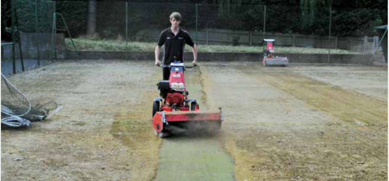
Above: The Kersten sweeper cuts through the mass of accumulated debris.
